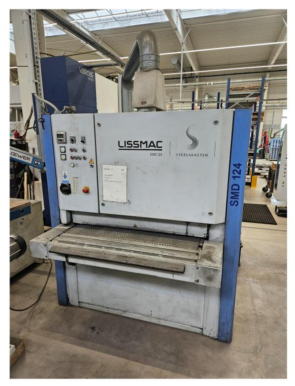
Deburring and finishing of laser cut and punched sheet metal parts.
